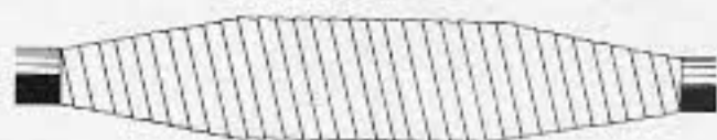
WRAP SEVERAL LAYERS OF TAPE WITH A 50% OVERLAP OVER THE CONNECTORS AND BUILT-UP JUNCTIONS. EACH OF THE LAYERS SHOULD BE WRAPPED IN REVERSE DIRECTIONS.
